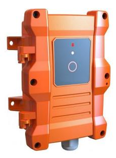
The Cirrus Dual Loop logger is a robust, low cost and sophisticated LTE/4G GSM logger with a wide range of input functions. This logger can operate on an external 12V supply or make use of standard alkaline batteries. It is well suited for applications such as those needed in the utilities industry or other remote measurement systems.
